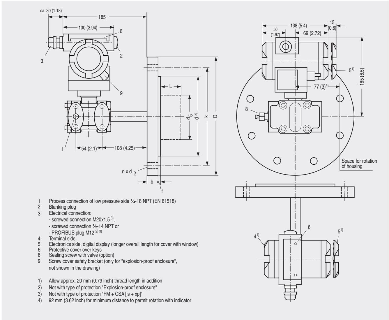
SITRANS P pressure transmitters, DS III PA series for level, including mounting flange, dimensions in mm (inch)
