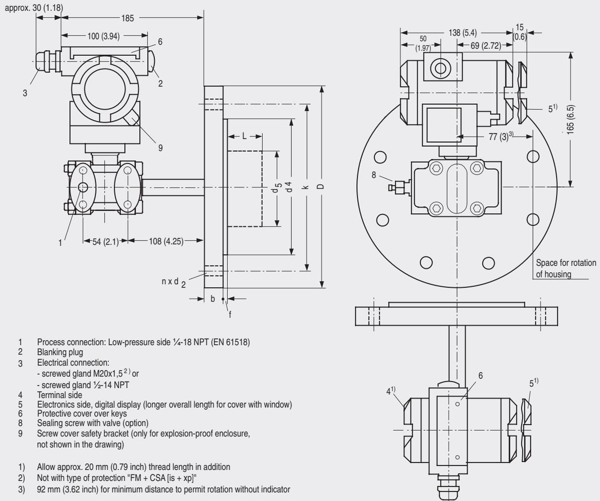
SITRANS P pressure transmitters, DS III FF series for level, including mounting flange, dimensional drawing, dimensions in mm (inch)
