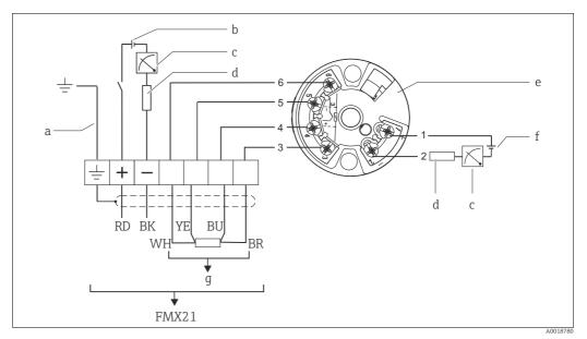
Waterpilot FMX21 with Pt100 and TMT182 temperature head transmitter (4 to 20 mA)  $^{\prime\prime}$  versions "NB" und "PT", feature 610 and 620 in the order code (  $\rightarrow$   $\triangle$  28)
