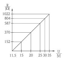
Temperature head transmitter TMT182 load chart for estimating the load resistance. Additional resistances have to be subtracted from the value calculated as shown in the equation.
