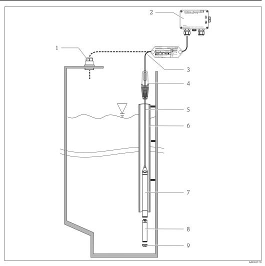
Installation examples, here illustrated with FMX21 with an outer diameter of 22 mm (0.87 in)
