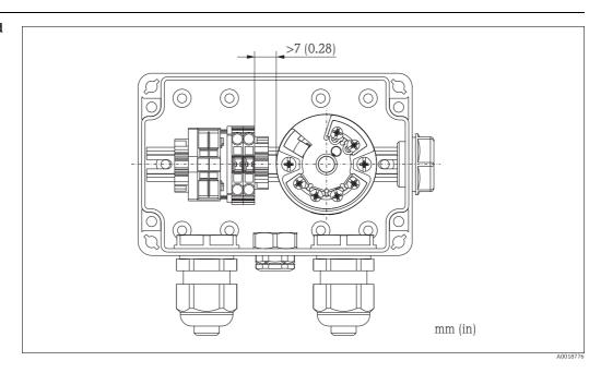
A distance of > 7 mm (> 0.28 in mm) must be maintained between the terminal strip and the TMT182 temperature head transmitter.
